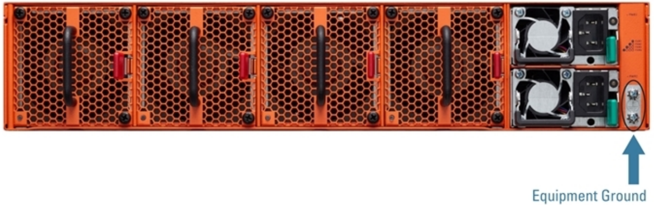
Figure 8 Ground Screws (GigaVUE TA Series-TA200 Shown)
