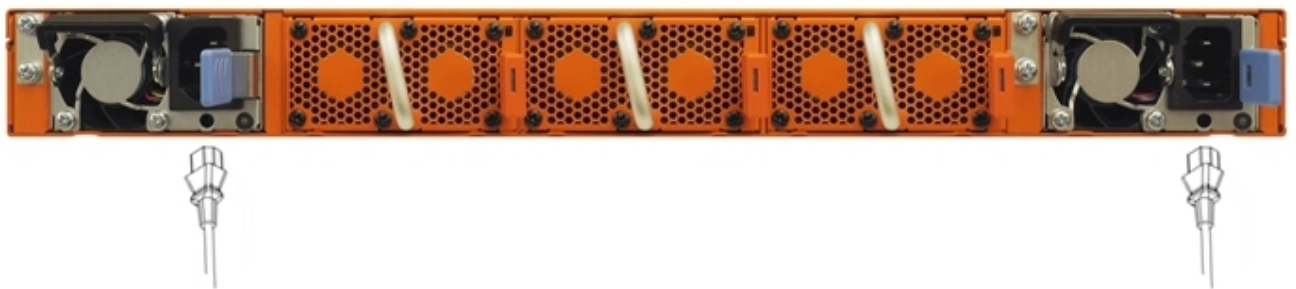
Figure 10 Connecting AC Power on a GigaVUE TA Series-TA100
